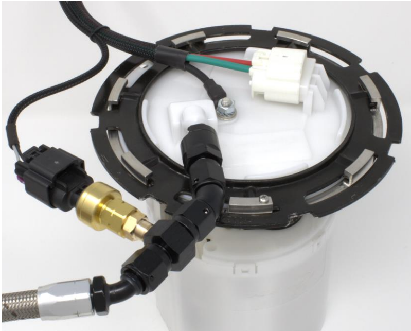
Photo 1. The fuel pressure sensor is installed into the fuel line near the outlet of the pump. The sensor may be mounted as far away as three feet from the pump. Do not mount the sensor near the engine. Wiring may route as needed to best fit into the car.
