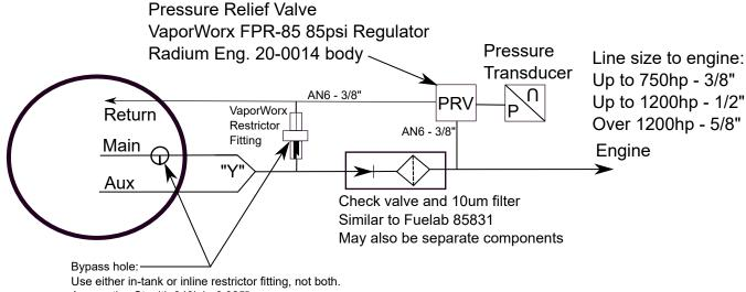
Aeromotive Stealth 340lph: 0.025" TI F90000267/274 450lph: 0.041" TI 90000285/295 525lph: 0.051"
