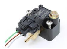
Photo 1. The MAP sensor wiring will need to be cut, stripped, and terminals installed as shown. P1 grey, P2 org/blk, P3 Lt green.
