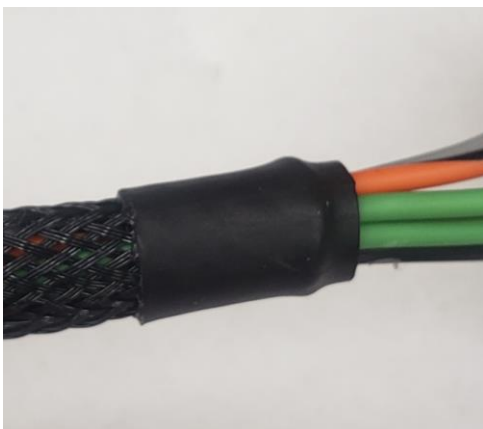
Photo 2. Note how the heat shrink covers the end of the braid to reduce fraying.
