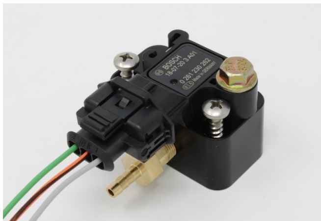
Photo 1 . Basic connection points for GM MAP sensors. Pin 1 = 5v Grey. Pin 2 = GND Or/Black. Pin 3 = Output Lt. Green
