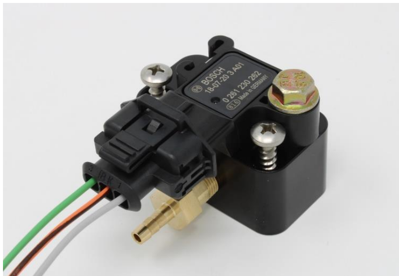
Photo 1. The assembled MAP sensor bracket. The rubber hose will attach to the barb fitting. The MAP sensor has a 4bar operating range.
