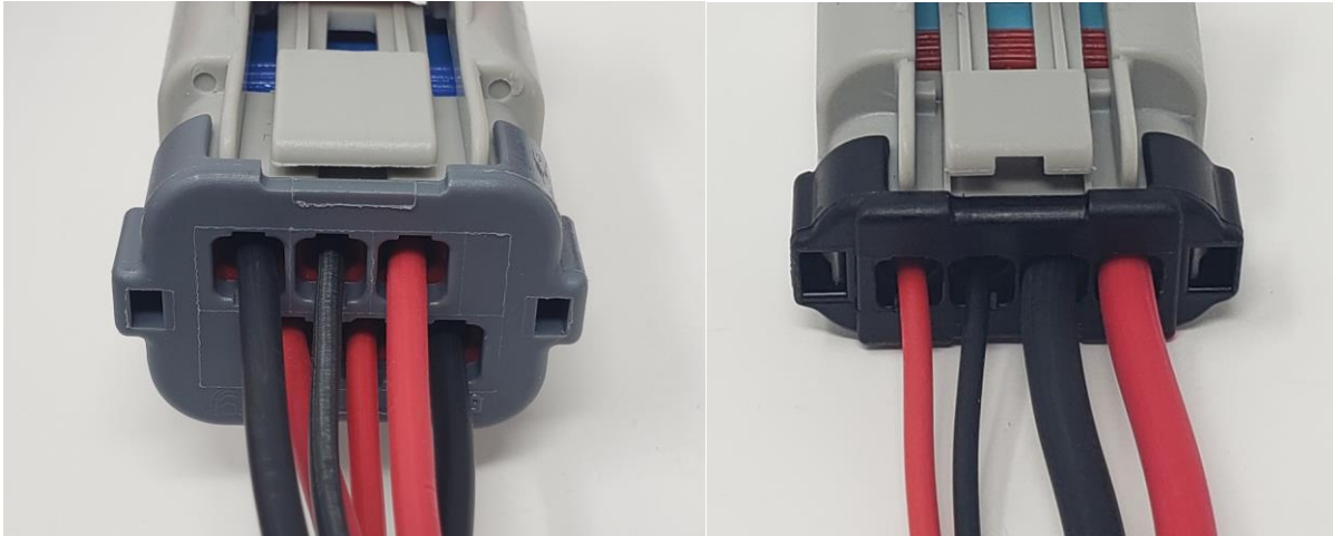
Photos 6/7. Left is the GT500 plug, right is the single pump module plug.
