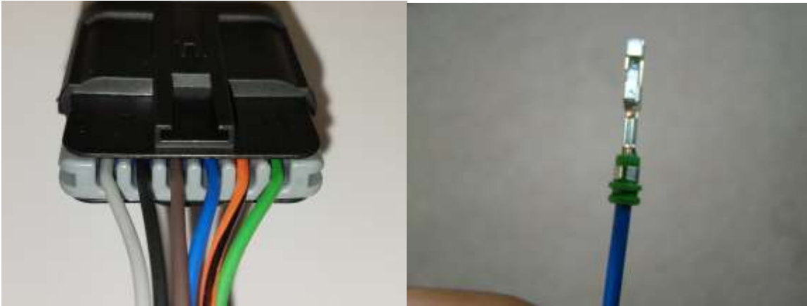
Photo 2: The GT150 connector body, terminals, seals, and terminal positional assurance clip. Photo 3: The terminal is crimped to the wire and seal. The Delphi terminal is P/N 12191818. The seal is 15366060.
