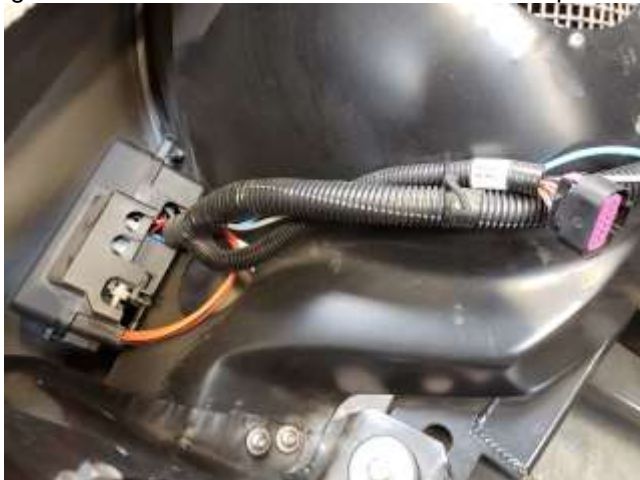
Photo 1: GM 12-pin bulkhead shown with purple cap. Extra terminals and seals are provided in the hardware kit to connect the tachometer, fused BAT and IGN power, etc.
