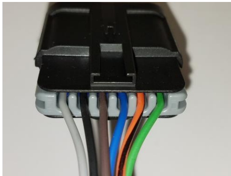
Photo 3: Delphi GT150 female connector (LH). Note that the colors align to each other on both plugs. Delphi designates the gender of the connector assembly by the terminal used, not the gender of the plug body. Hence the plug that appears male uses a female terminal, and is designated female by Delphi.
