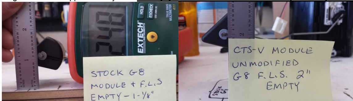
Photos 1 and 2. Empty float height readings for Pontiac G8 / CTS-V fuel modules.
