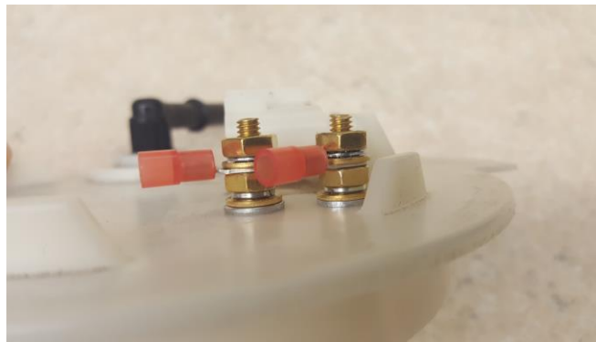
Photo 3. The stack assembly. Fuel level sensor wiring not yet connected.
