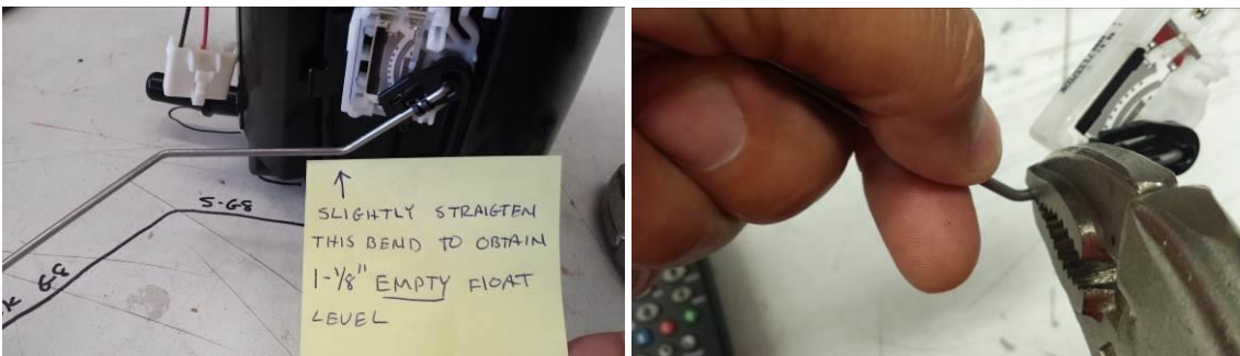
Photos 5 and 6. Make the bend along the same axis as the OE bend. Do not allow bending loads to travel up to the fuel level sensor body.
