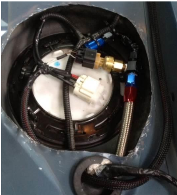
Photo 6. Note the how the woven braid routes through the OE grommet and then goes to the other side of the car. The pressure sensor must be placed near the outlet of the fuel module.
