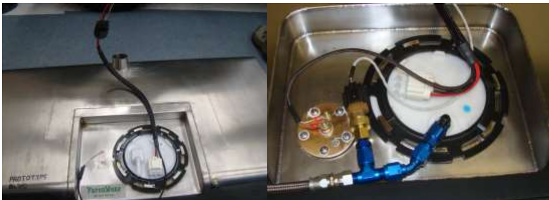
Photo 4 and 5. Note the black GT280 four-pin connector. Route the harness along the top of the tank to a convenient location, such as behind the license plate. The fuel pressure sensor can often be placed in the recess of the tank, providing protection and making for a clean installation.
