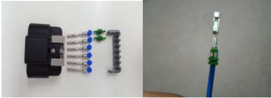
Photo 1: The GT150 connector body, terminals, seals, and terminal positional assurance clip. Photo 2. The terminal is crimped to the wire and seal. The part number for the Delphi terminal is 12191818. The seal is 15366060. Spare parts are available from Vaporworx.
