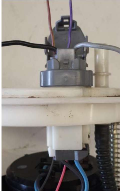
Photo 15. OE G8 fuel module wiring. Note the violet lines up with the FLS pink wire, the brown to the black FLS wire, and the grey wire that will run to the VaporWorx grey wire in the three-pin Molex connector.
