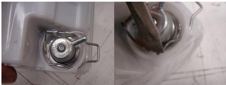
Photo 3/4: The new regulator is inserted, the ground strap installed, and the retaining wire partially seated. The ends of the wire are close to the holes/slots in the fuel module body. The wire head and ends must fully seat into the holes/slots and the wire must surround the regulator body.
