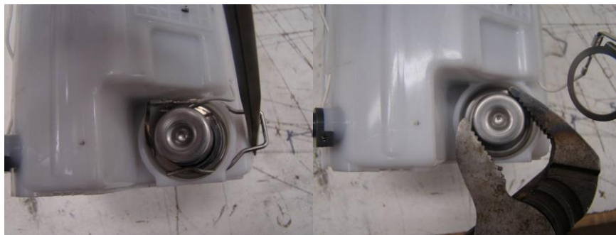
Photo 1/2: Note the ground strap ring that is located under the retaining wire. Do not use excessive force. Photo 2: Note the ground strap has been pushed aside. There are no internal parts that retain the fuel pressure regulator.
