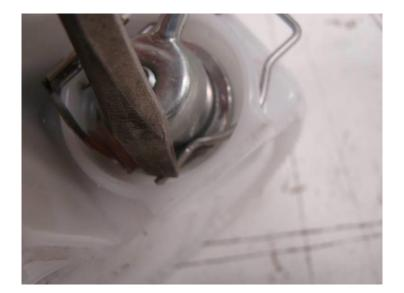
Photo 7: In some cases it may be necessary to push down on the end of the retaining wire ends to align them to the holes/slots in the module body. Take care to keep the ground wire under the retaining wire.STEP 6: Fully seat the retaining wire. After seating use a pair of needle nose pliers to squeeze the wire ends together, making them fit the body of the regulator better, as seen in Photo 8. It may be necessary to slightly bend the wire near the wire head to obtain good fitment.
