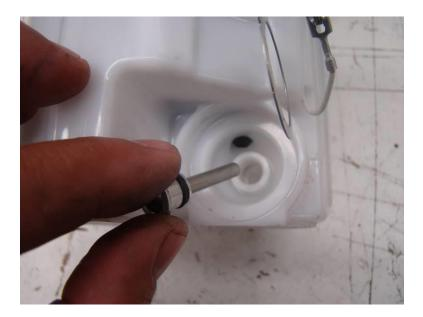
Photo 3: Insert the FPRAGM5 into the small hole until fully seated. If the fuel filter interferes with easy installation use a Philips screwdriver to move to the side (left in the photo.)
