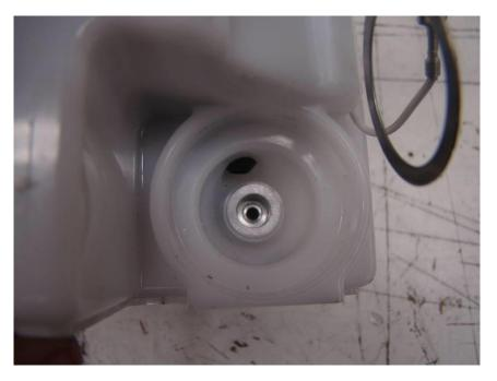
Photo 4: The FPRA is fully seated in the fuel module.
