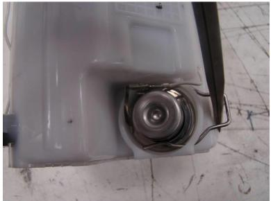
Photo 1: Note the ground strap ring that is located under the retaining ring. Do not use excessive force.
