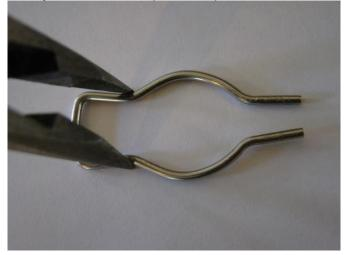
Photo 6A. Bend the retaining clip so that the points of the clip are  $\frac{1}{4}$ " apart when not compressed by the needle-nose pliers.
