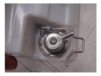
Photo 6b: The new regulator is inserted, the ground strap installed, and the retaining wire partially seated. The ends of the wire are close to the holes/slots in the fuel module body. The ends must go into the holes/slots.
