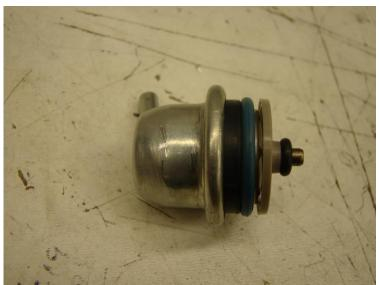
Photo 5: The ready-to-install fuel pressure regulator.
