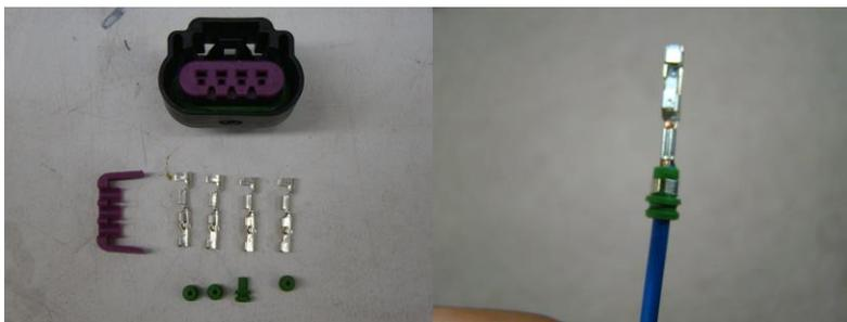
Photo 1: The GT150 connector body, terminals, seals, and terminal positional assurance clip. Six cavity PressureWorx plug similar. Photo 2. The terminal is crimped to the wire and seal. The part number for the Delphi terminal is 12191818. The seal is 15366060.
