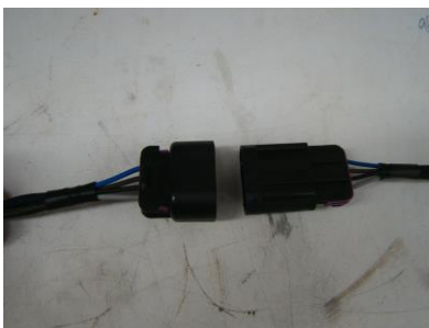
Photo 3: Delphi GT150 female connector (LH). Note that the colors align to each other on both plugs.
