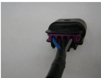
Photo 4: The purple terminal position assurance clip is installed. Six cavity plug similar.
