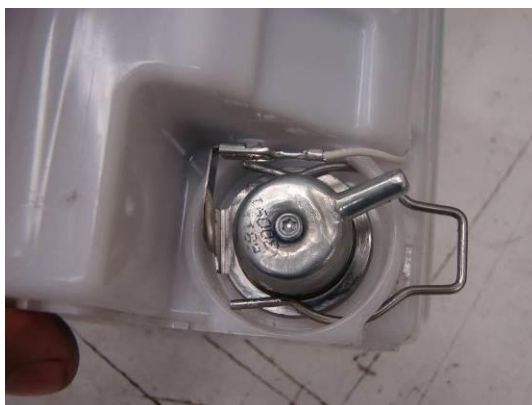
Photo 6b: The new regulator is inserted, the ground strap installed, and the retaining wire partially seated. The ends of the wire are close to the holes/slots in the fuel module body. The ends must go into the holes/slots.
