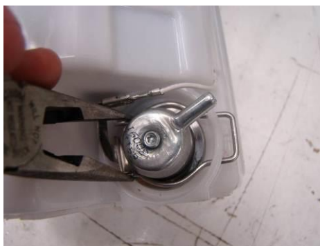
Photo 8: Squeeze the ends of the retaining wire together to help fit them to the regulator body. When complete the head of the retaining wire will be seated against the fuel module.
