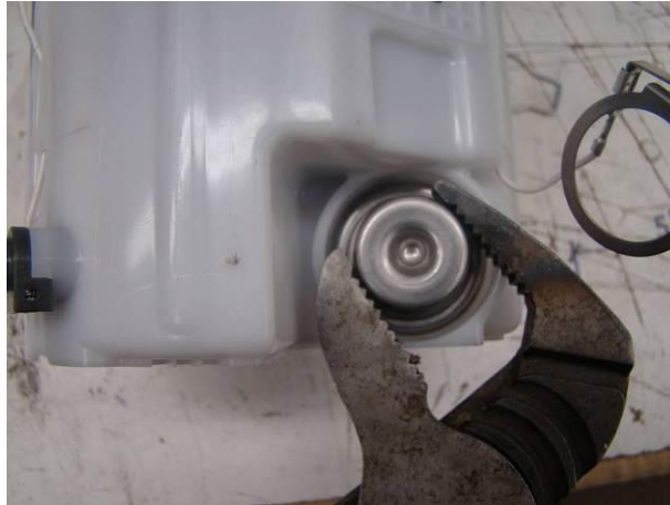
Photo 2: Note the grounding ring has been pushed aside. There are no internal parts that retain the fuel pressure regulator.
