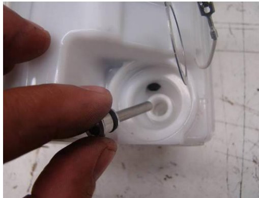
Photo 3: Insert the FPRAGM5 into the small hole until fully seated. If the fuel filter interferes with easy installation use a Philips screwdriver to move to the side (left in the photo.)
