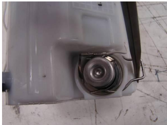
Photo 1: Note the ground strap ring that is located under the retaining wire. Do not use excessive force.
