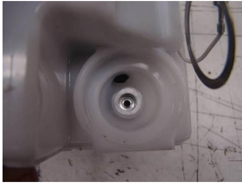
Photo 4: The FPRA is fully seated in the fuel module.
