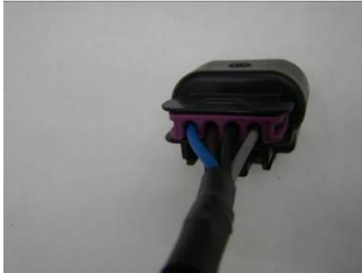
Photo 4: The purple terminal position assurance clip is installed. Six cavity plug similar.
