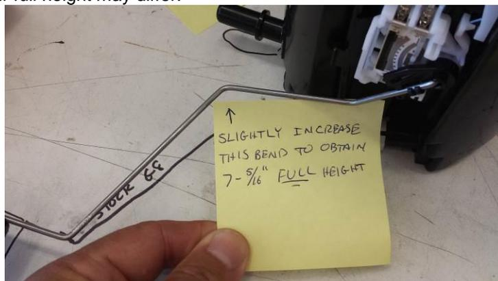
Photo 7. Full float height bend adjustment. Make the bend along the same axis as the OE bend.
