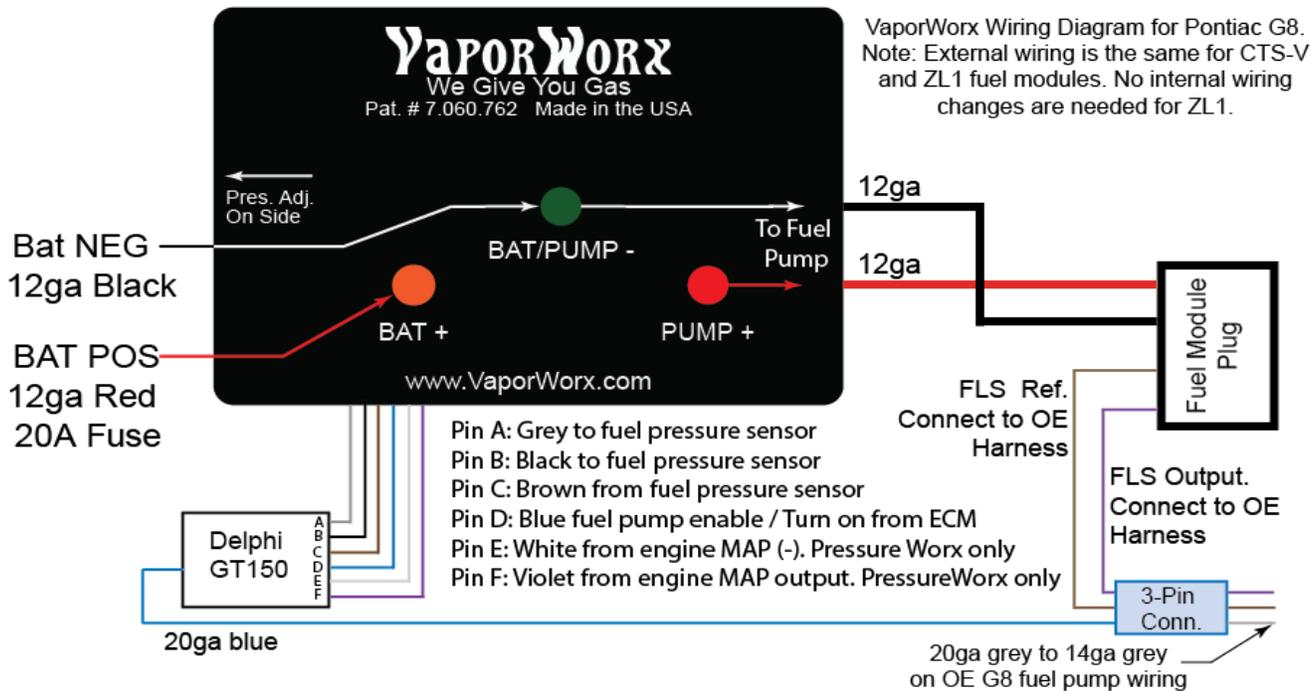
Diagram 1. Basic wiring layout for the VaporWorx controller. The wiring may enter/exit the controller area as needed provided that there is no chance of shorting between connections.
