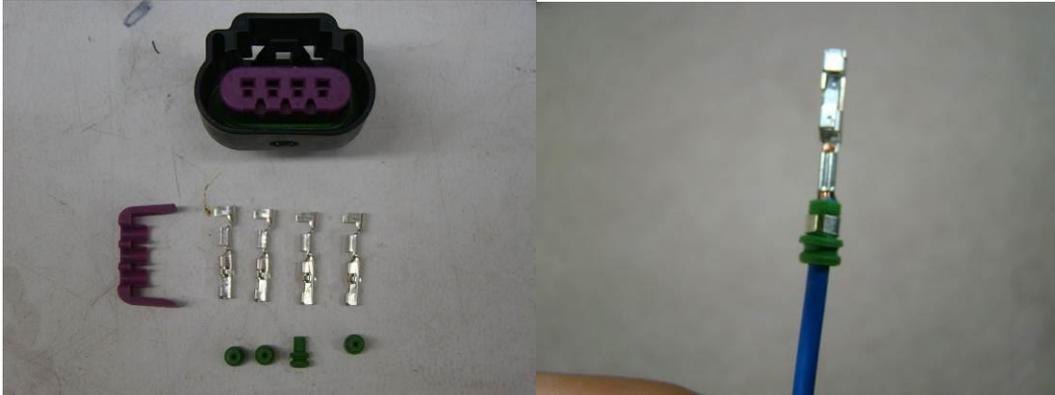
Photo 17: The GT150 connector body, terminals, seals, and terminal positional assurance clip. Six cavity PressureWorx plug similar. Photo 18. The terminal is crimped to the wire and seal. The part number for the Delphi terminal is 12191818. The seal is 15366060.
