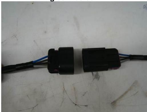
Photo 19: Delphi GT150 female connector (LH). Note that the colors align to each other on both plugs. Delphi designates the gender of the connector by the terminal used. Six pin plug similar.
