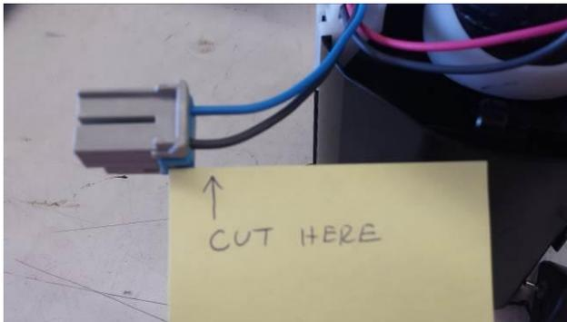
Photos 8: Cut wires near plug body.
