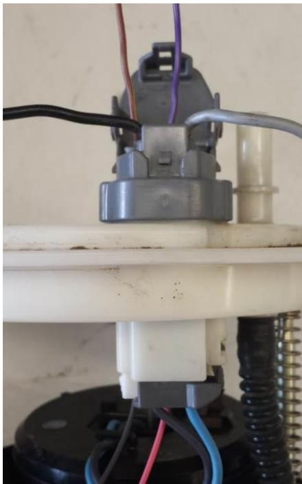
Photo 15. OE G8 fuel module wiring. Note the violet lines up with the FLS pink wire, the brown to the black FLS wire, and the grey wire that will run to the VaporWorx grey wire in the three-pin VaporWorx harness connector.
