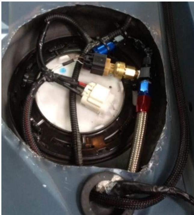
Photo 16. Note the how the woven braid routes through the OE grommet and then goes to the other side of the car. The VaporWorx controller is mounted near the battery, so route the wiring to best suit the layout of the car. The fuel pressure sensor wiring can also be included.
