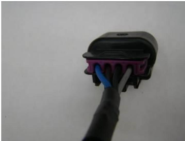
Photo 21: The purple terminal position assurance clip is installed. Eight cavity plug similar.
