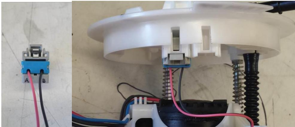
Photos 10 and 11. Plug and final installation arrangements.
