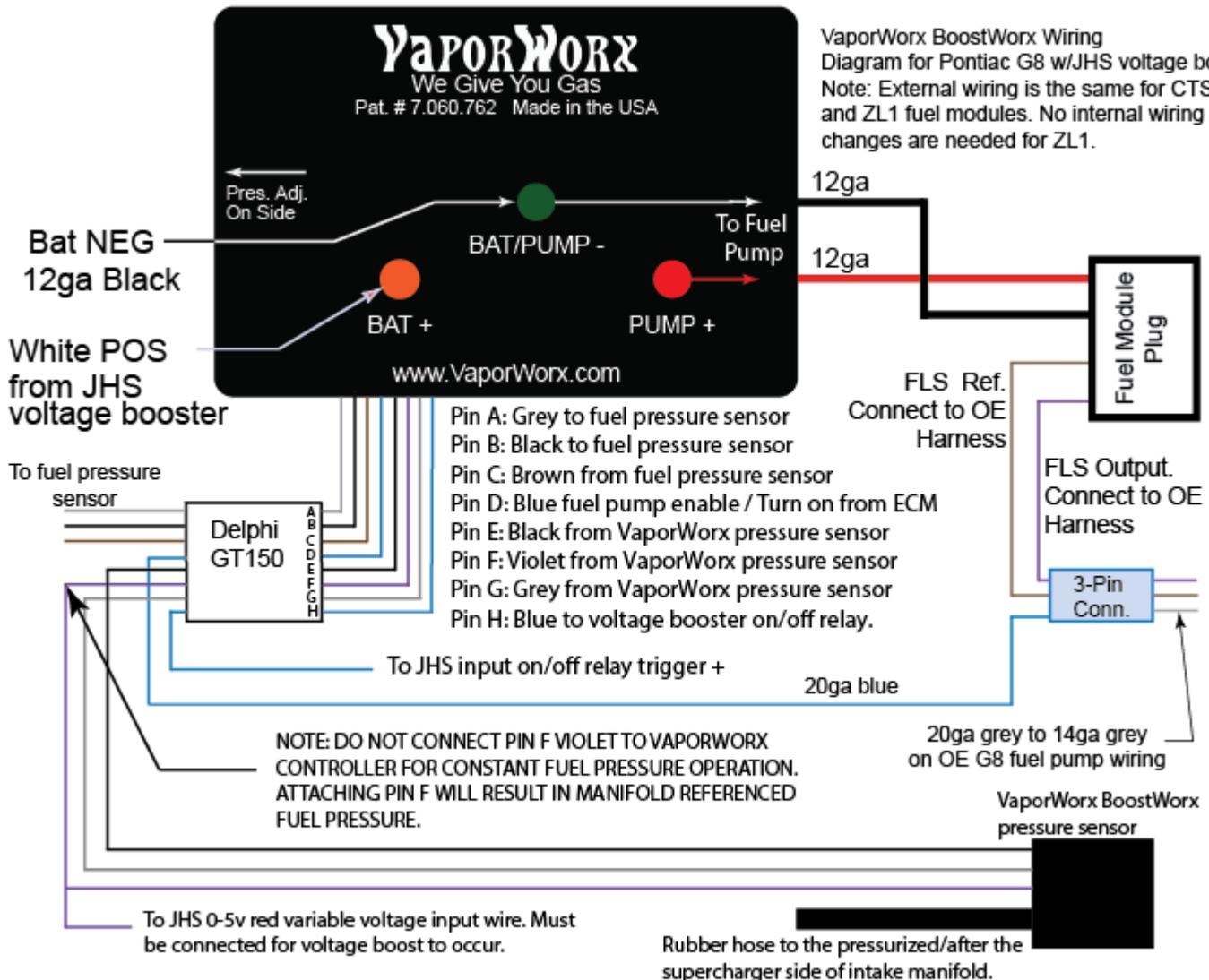
Diagram 1. Basic wiring layout for the VaporWorx BoostWorx G8 controller. The wiring may enter/exit the controller area as needed provided that there is no chance of shorting between connections.
