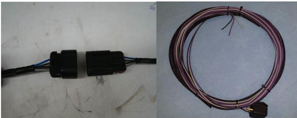
Photo 19 and 20: Delphi GT150 female connector (LH). Note that the colors align to each other on both plugs. Delphi designates the gender of the connector by the terminal used. Six/eight pin plug similar. BoostWorx pressure sensor (RH) harness. Note the three wires that route to the VaporWorx control box and the brass manifold connection.
