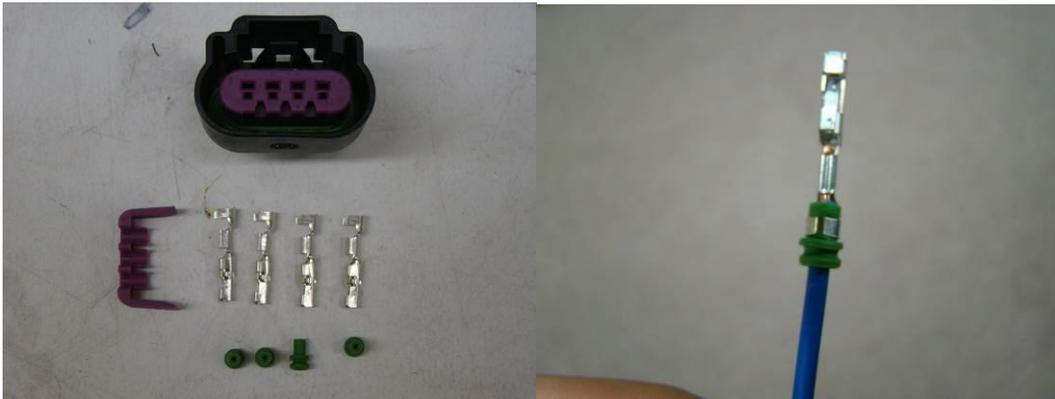
Photo 17 and 18: The GT150 connector body, terminals, seals, and terminal positional assurance clip. Eight cavity plug similar. The terminal is crimped to the wire and seal.
