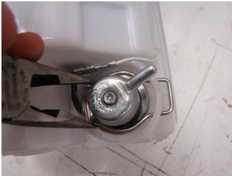
Photo 8: Squeeze the ends of the retaining wire together to help fit them to the regulator body. When complete the head of the retaining wire will be seated against the fuel module.
