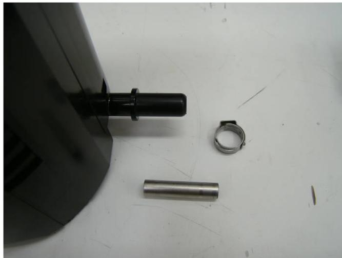
Photo 1. The uncut venturi pump pickup tube is shown along with the 5/16" tube and Odiker clamp.
