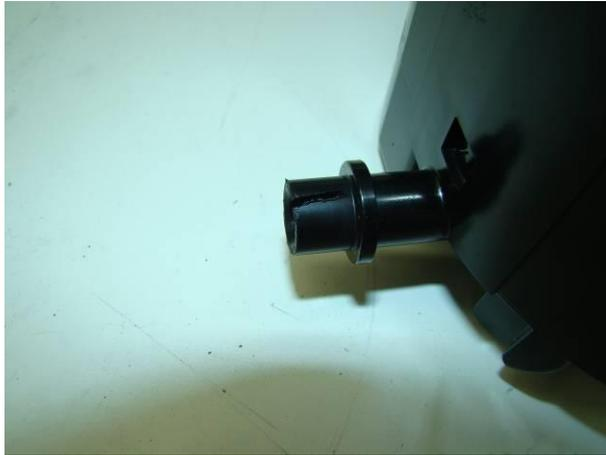
Photo 2. The venturi pump pickup tube has been cut radially and axially. The tube has also been drilled to  $21/64$ " to a depth of 1". The tube bore can also be chamfered.
